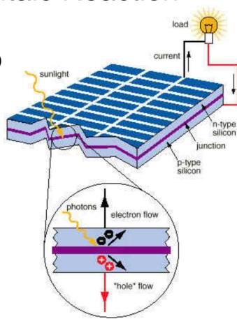
Two layers of silicon produce a positive and negative energy flow, separated by the junction material.
